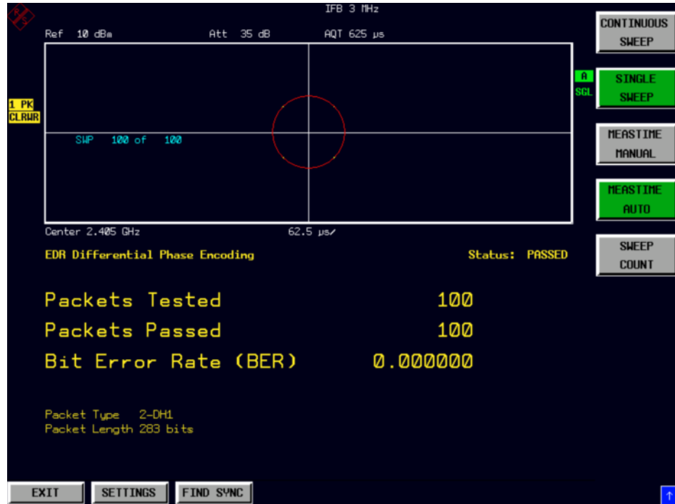
Fig. 3-13 Differential Phase Encoding (EDR) measurement
